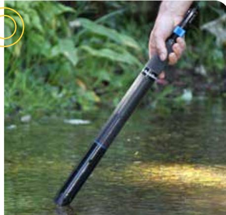
This means it is ideal for discrete long term deployment, using only a Kevlar deployment cord without the need for cables or auxiliary equipment at ground level. The Maji-Sonde measures the 10 standard parameters and has the ability to add up to 6 unrestricted additional electrodes.
