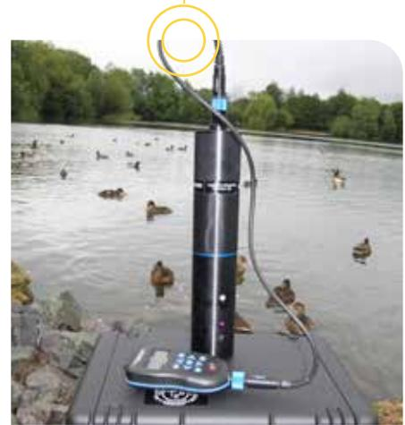
To carry out water quality analysis the probe is simply lowered into the water and the results are displayed on the hand-held device. The meter has inbuilt GPS to record the exact location in which the results were taken and has the capacity to store over 1000 data sets.
