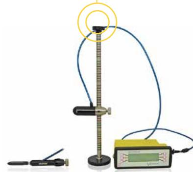
Two sensor types are available to suit different application requirements. One for measuring speeds in water depths of 15cm or more and one for 5cm or more. Both offer excellent durability, reliable accurate data and are suitable for use in clean water and dirty or difficult environments. Both instruments are calibrated to NAMAS traceable standards for speeds up to 1m/s.
