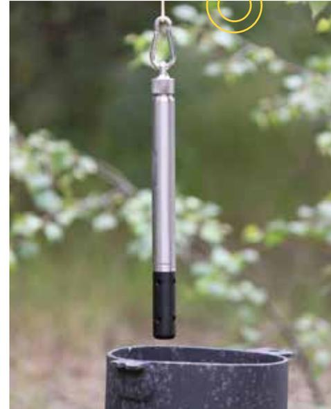
The logger collects data at user-defined intervals and stores the information in its internal memory – it can take up to 1 reading per second and store up to 500,000 readings at once. Made from titanium, the logger is built for deployment in all environments from fresh groundwater to salty marine waters. To download the recorded data, simply retrieve the logger and connect it to a PC or a handheld GPS meter.
