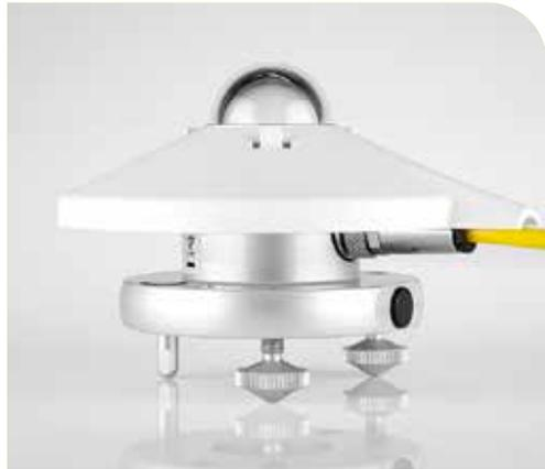
The SMP3 is a thermopile pyranometer, which differs from the technology used in the SCP which is a silicon-cell pyranometer. The difference is that silicon-cell pyranometers have high errors in cloudy conditions, whereas thermopile pyranometers have a much broader and more uniform spectral response, meaning they perform well in all weather conditions.
