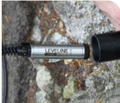
The LL-MINI is a water level and temperature sensor that provides accurate and reliable data with minimal maintenance. It is constructed using titanium and features sensitive pressure and temperature sensors. It outputs directly in SDI-12 or Modbus (RS-485) meaning you can connect it to any SDI-12 ready logging device. It has no internal power or memory, it's simply a sensor that will send data to your chosen logging device.
