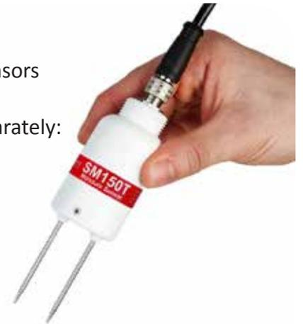
The SM150T measures soil moisture and temperature with research-grade accuracy. It offers stable, robust and reliable performance at a great price. The advanced patented electronics and tough build quality produce a highly reliable soil moisture sensor with exceptional salinity and temperature stability. The SM150T is engineered to withstand long term burial – the sensor, connectors and cable are all environmentally protected to IP68.
