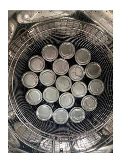
Once sterilization or pasteurization phase is finished, a fast cooling cycle begins, which lowers temperature through a water shower and water immersion system.
