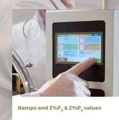
Experienced users can customise pressure support and temperature ramps before and after thermal processing. The actual  $\Sigma\%F_0$  and Σ%P<sub>o</sub> values achieved are also displayed on screen and presented in the reports.
