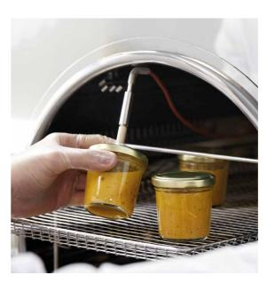
By using a temperature probe placed inside a product sample, we ensure a perfect control of the process, ensuring the correct elimination of all microbial life within each container, while also preserving the organoleptic properties and minimizing possible changes regarding the nutritional value of the packaged product.
